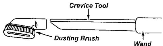
An extra wand, without tabs, is included. This extra wand can be added to the wand with tabs for extra reach. Insert wand and twist a quarter of a turn to secure fit.
